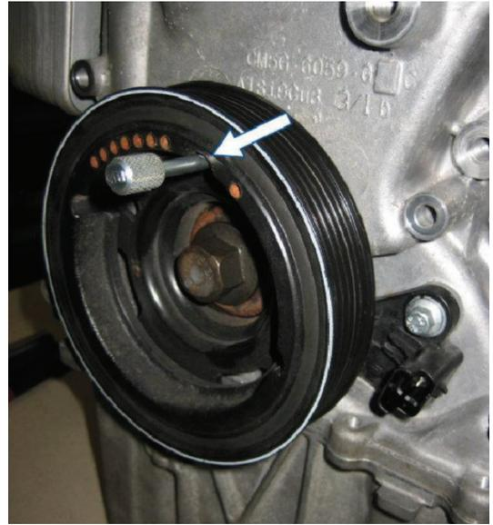
Remove the tool (3) and refit the crankshaft blanking plug.
