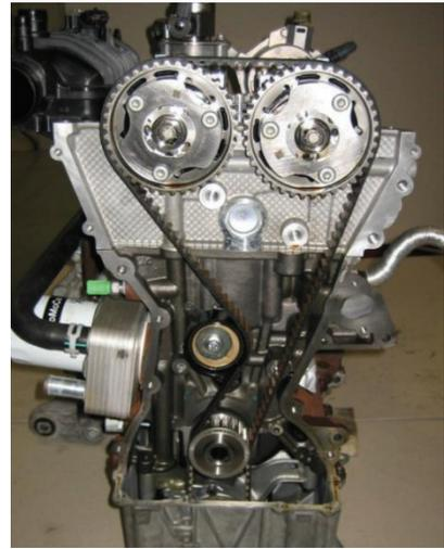
Loosely position correct one tool (1) on to the Inlet camshaft and the other tool (1) on to the Exhaust camshaft. Tighten locking screws of the camshaft tools finger tight only, ensuring that the camshaft tools are positioned correctly on the camshafts. Secure the camshaft tools to the cylinder head by tightening the 8 retaining bolts to 10 Nm.
