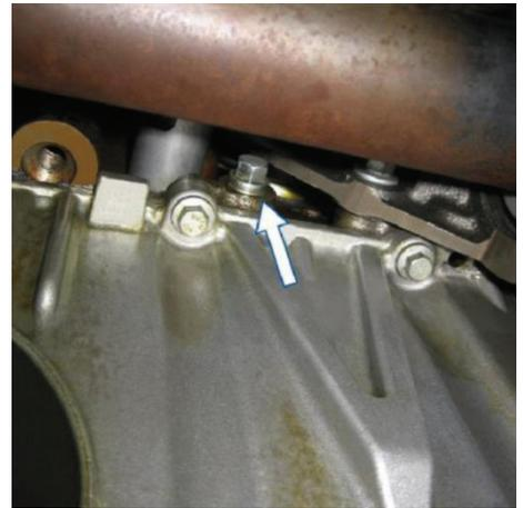
Fit tool (3), ensuring that it is fully located in the engine block.
