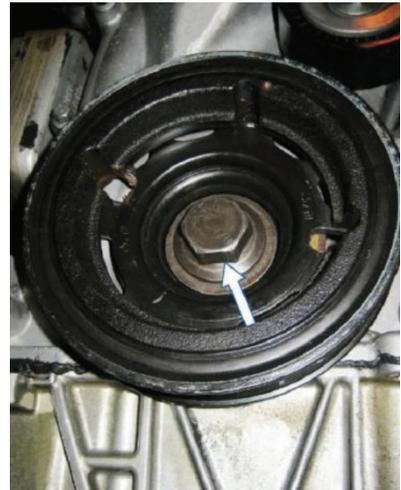
Remove the crankshaft pulley and remove the crankshaft oil seal from the timing belt cover, taking care not to damage the sealing face of the cover.
