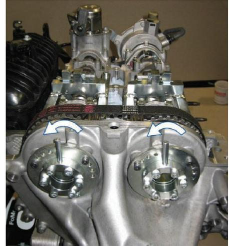
Using a new bolt, fit the crankshaft pulley into the crankshaft, finger tight only at this stage. Take care not to damage the reluctor ring on the rear of the crankshaft pulley. Ensure that the alignment hole of the pulley is positioned at approximately at 10 o'clock relative to the pulley central bolt. Insert tool (6) through the alignment hole in the pulley and into the alignment hole on the engine block.
