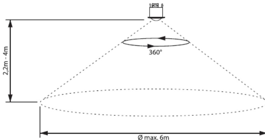
(UK) The detection range of the motion detector is approx. 6m and 360° (free area) at a mounting height of 2.2-4m at the ceiling. In closed rooms the detection distance can be lower, according to room layout. .
