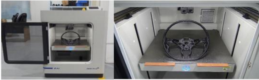
Steering Wheel Printing Process
