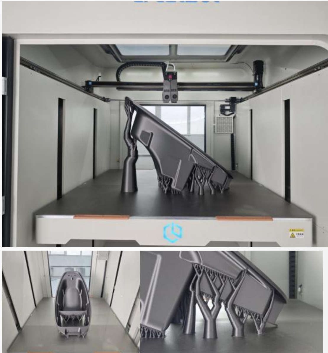
Electric Scooter Base Printing Details@CreatBot
