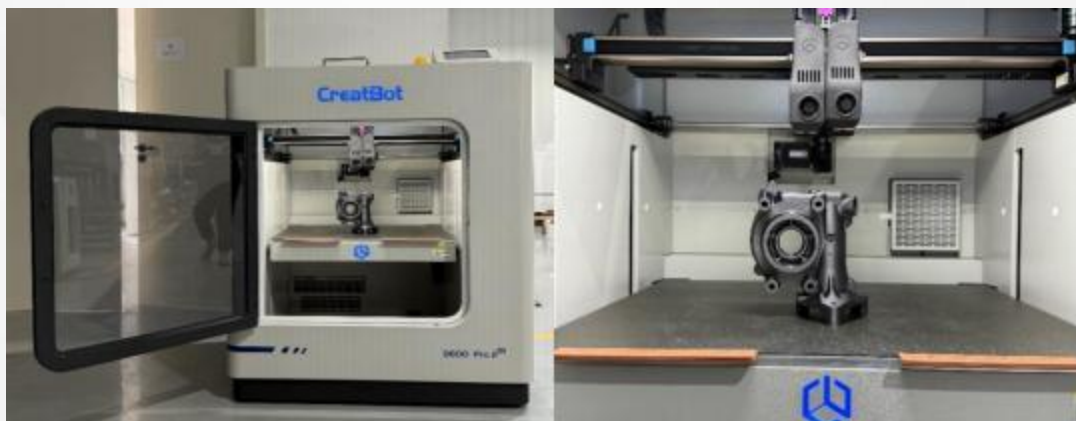
Oil Pump Housing Model 3D Printed by Bosch Using CreafBot D600 Pro2 HS
