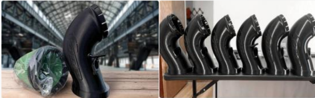
Batch manufacturing of 3D-printed intake pipes
