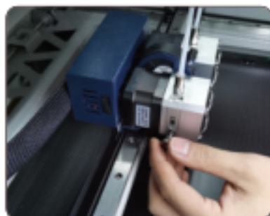
Tighten pressure nut
