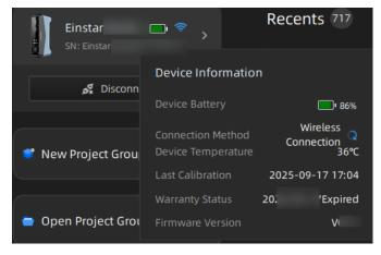
Once the device is successfully connected, the information about the device will be displayed in the top left corner; click > to view more detailed device information.
