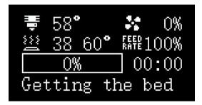
The print will start after the components reached the printing temperature.
