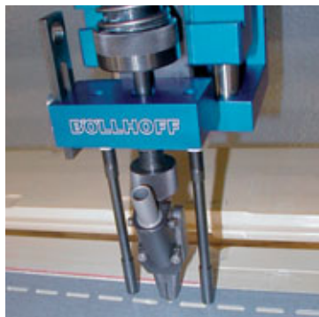
Vorschraubung in Holz Screw fastening into wood
