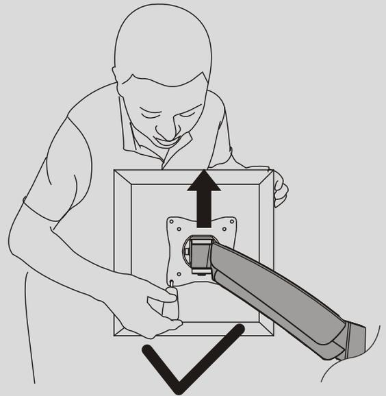
**Attention:** The arm can shoot up upwards because of the gas pressure spring!
