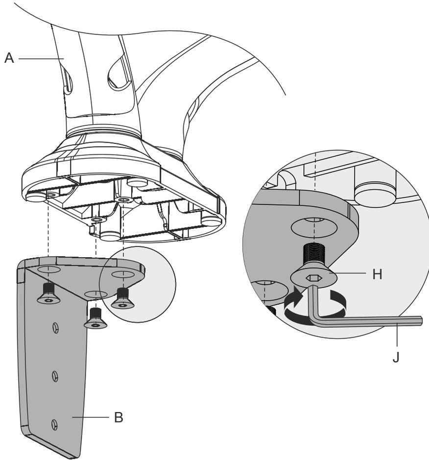
Variation 1: For desktop thickness: min. 10mm - max. 55mm
