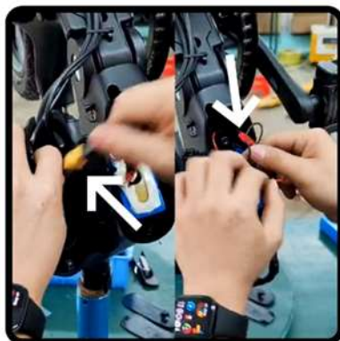
11. Unplug two power Cables.
