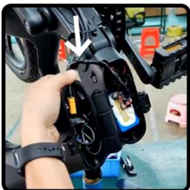
16. Arrange the wiring harness neatly .
