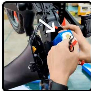
12. Gently remove the battery.
