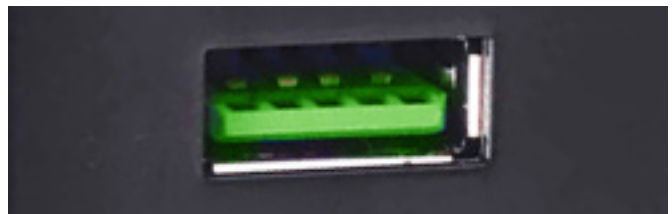
USB – Ladebuchse (max. 1A 5V DC)
